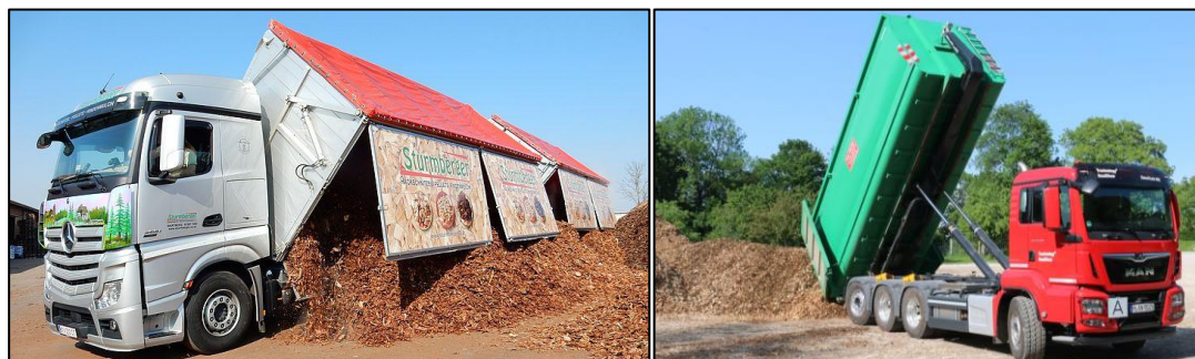
Figure 37. Truck 34 unloading techniques for an interim storage facility at the port in Walvis Bay 35
