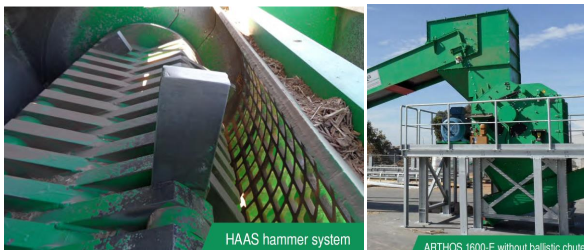
Figure 16. HAAS Hammer system and the hammer mill ARTHOS 1600 E 19
