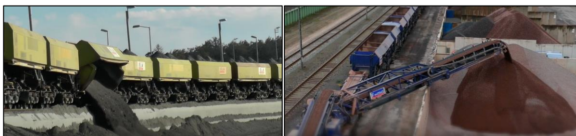
Figure 36. Locomotive unloading techniques 32 for an interim storage facility at the port in Walvis Bay 33
